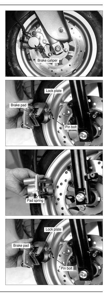
Install the brake caliper into the right front fork.
