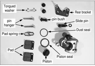
Apply the silicone grease to the pin bush.
