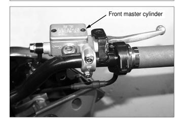
Inatall the brake hose to the master cylinder with 2 new sealing washers and the hose bolt. Torque: 3.5kgf • m
