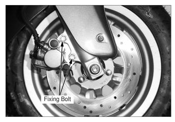
Remove the brake caliper from the right front fork.
